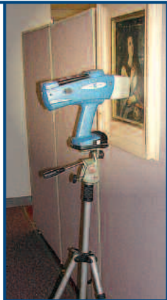
The Innov-X analyzer may be remotely controlled from a tripod to examine paintings and other art without the analyzer touching the artwork.
